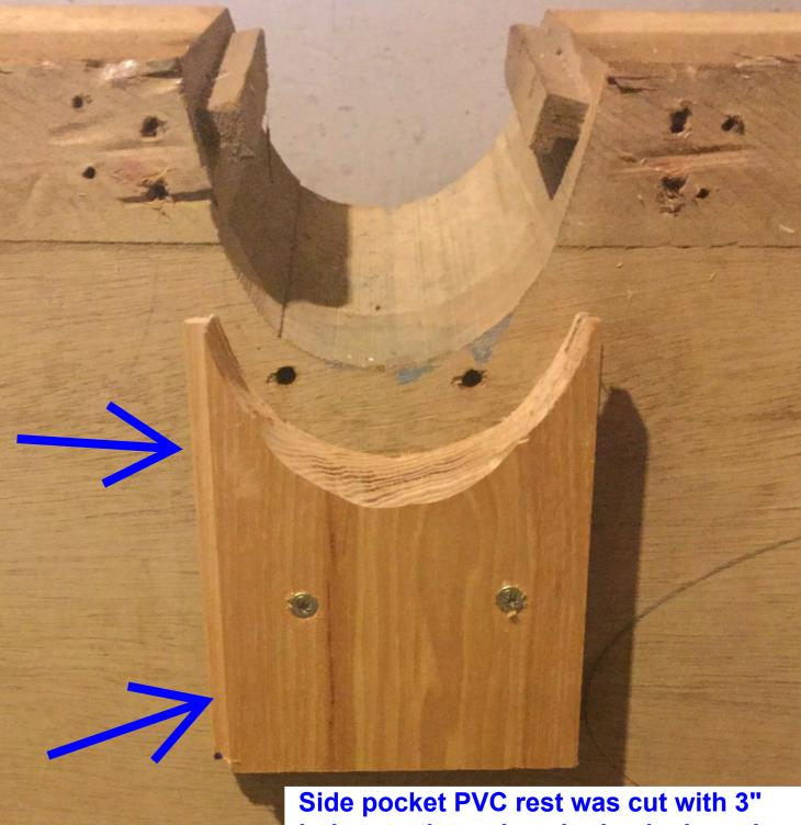
Side pocket PVC rest was cut with 3" hole saw through a single plank, and then halved yielding 2 semicircled rests. Arc was angulated with drum sander and Dremel.
