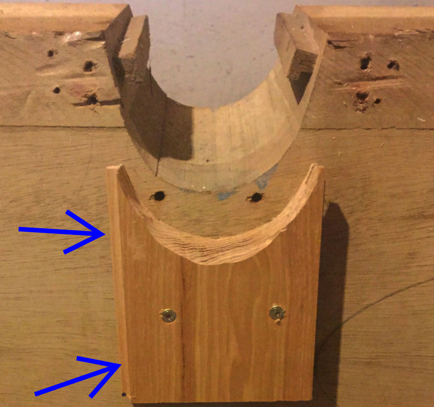
Side pocket PVC rest was cut with 3" hole saw through a single plank, and then halved yielding 2 semicircled rests. Arc was angulated with drum sander and Dremel.
